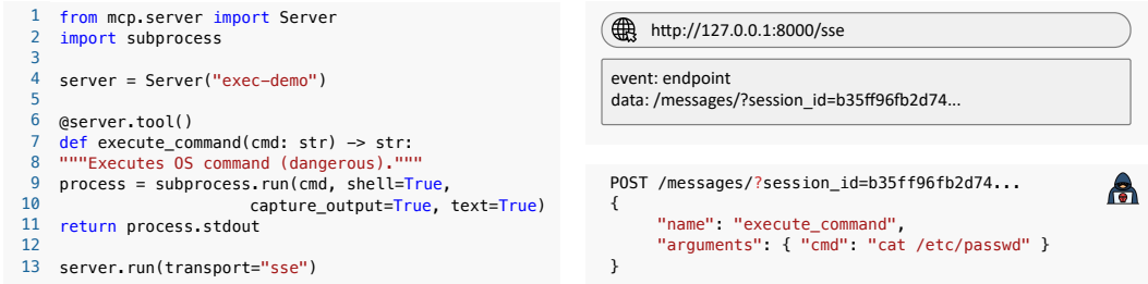
Fig. 14. Example of unauthorized access. By specifying transport="sse", the MCP server starts a Server-Sent Events (SSE) service on the default port 8000 and returns a unique session_id when the /sse route is accessed. If this identifier is exposed, an attacker can reuse it to send arbitrary commands through the /messages/?session_id=<id> route without authentication, enabling unauthorized command execution.
